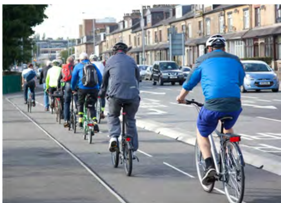
Figure 28 – Fully segregated two-way cycle track (Leeds)
