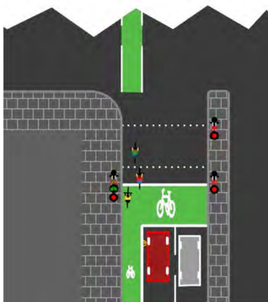
Figure 34 – Diagram of early release signal for cycle users
