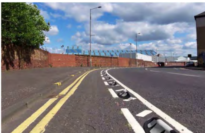
Figure 30 – Cycle lane with light segregation
